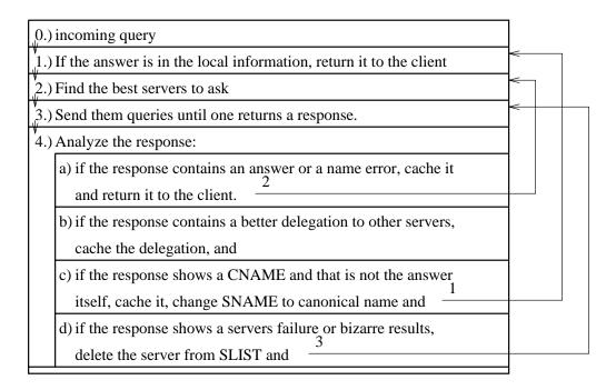
Figure 2.8 Resolver algorithm
