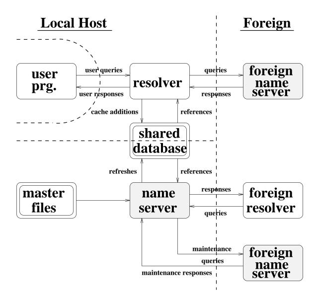
Figure 2.9 Data flow between DNS entities
